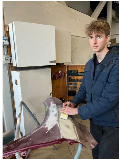
Auto body10 - dent repair on fenders
